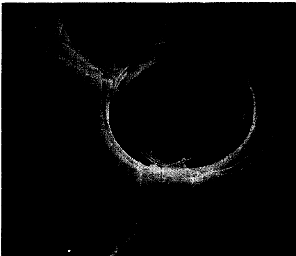
FIG. 1. Scanning micrograph of a pit produced by platinum-catalyzed oxidation of graphite in 5 Torr O_2 at 500^\circ C ; \times 2070 .
